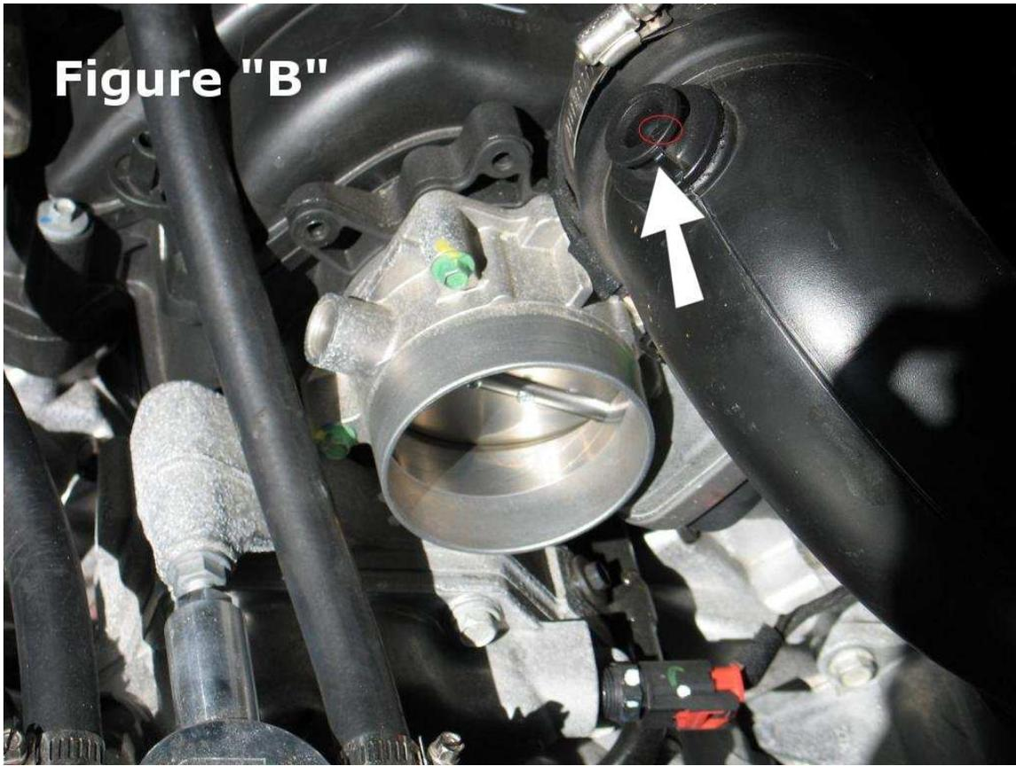
Next unscrew the clamp on the tube at the throttle body and remove the single bolt holding the airbox to the engine compartment as shown in (figure "C").
