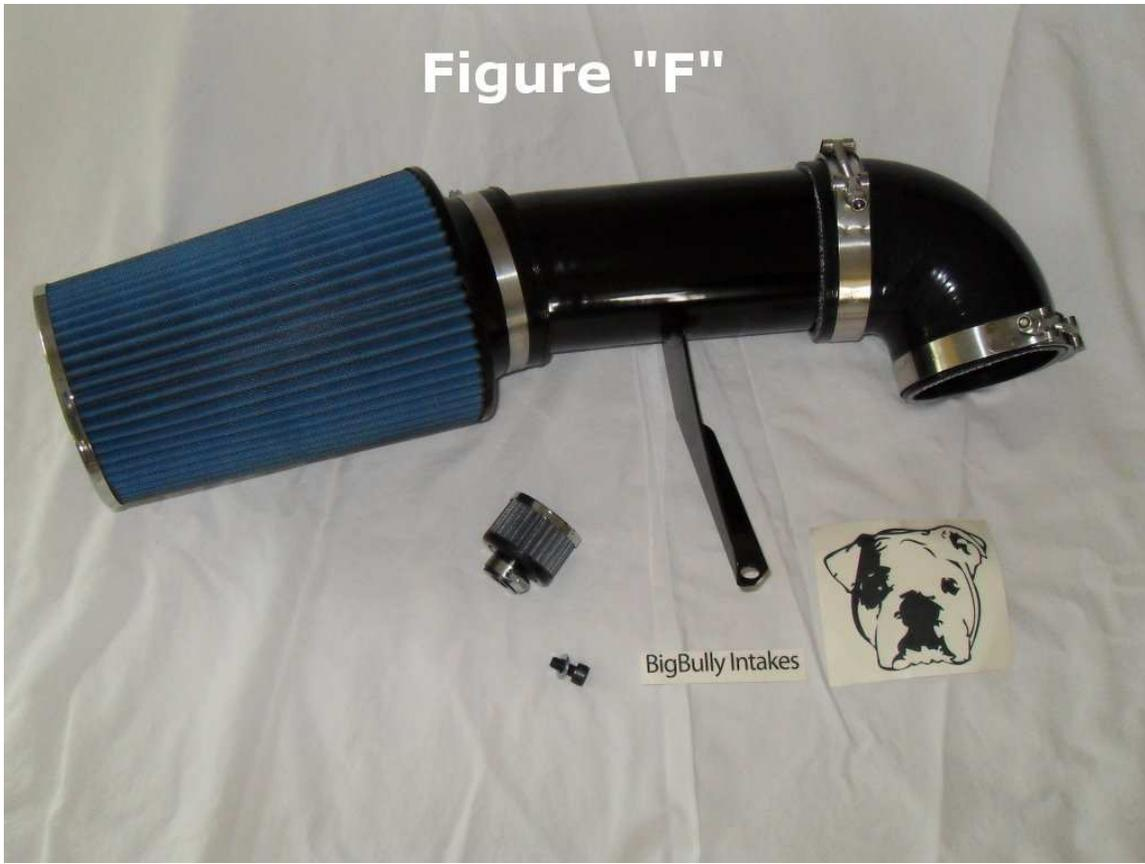
Next line up the mounting bracket on the cold air intake tube with the mount on the engine. Insert the provided M8x125x5/8" stainless steel bolt and 5/8" stainless steel washer as shown in (figure "G").
