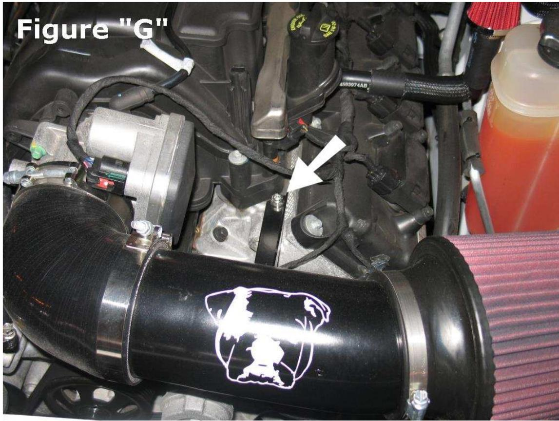
Use an Allen wrench to tighten the bolt. (Don't forget the washer). Tighten loose do not over tighten yet so you can move or rotate the tube into its final position
